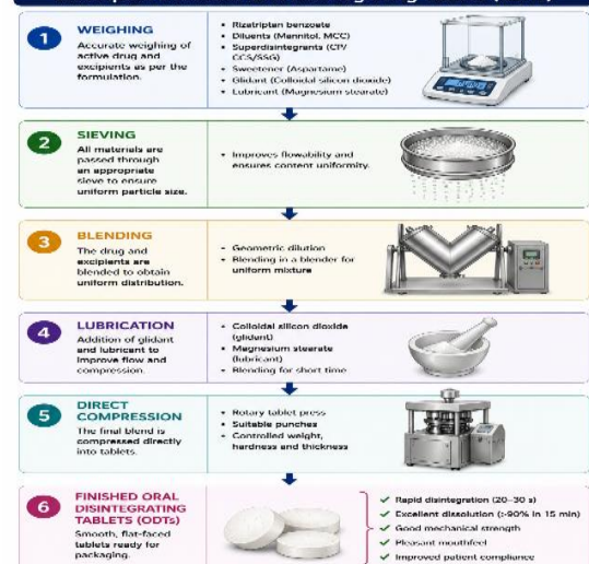
Figure 4. Manufacturing Process of Rizatriptan Benzoate Oral Disintegrating Tablets (ODTs)
