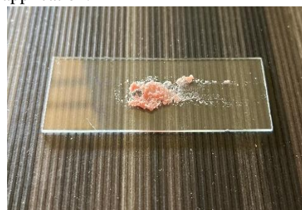
Figure 4: Spreadability of lip balm at room temperature G - Good: uniform, no fragmentation; perfect application, without deformation of the lip balm.
