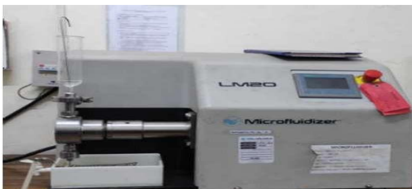
Figure 1: Microfluidizer used in the formulation of Flurbiprofen-loaded Nanoemulsion Characterization of Nanoemulsion
