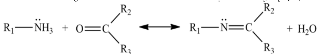
Scheme1: General scheme for Schiff base reaction.
